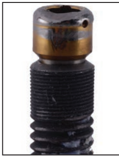
Fig. 7 — Low profile abutment that caused the implant loss
