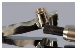
Polishing small parts around connections
