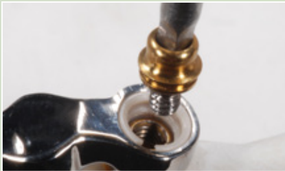
Insertion of the Ot Equator seeger inside the self-extracting peek ring already in position.
