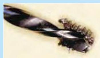
BROKEN SCREW BEING REMOVED
