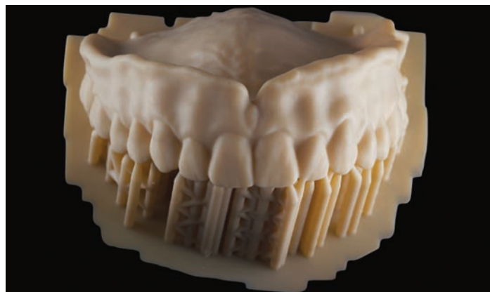
Fig. 8 — The prototype obtained with a 3D printer
