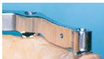
Locking key in position without spacer rings
