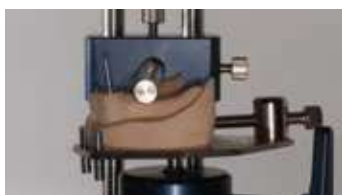
Model analysis using the Rhein83 Parallelometer
