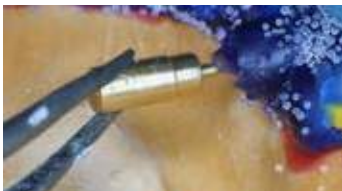
Pull out the brass positioner and cast.
