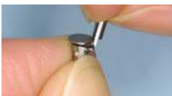
Bend the locking key and brake it.
